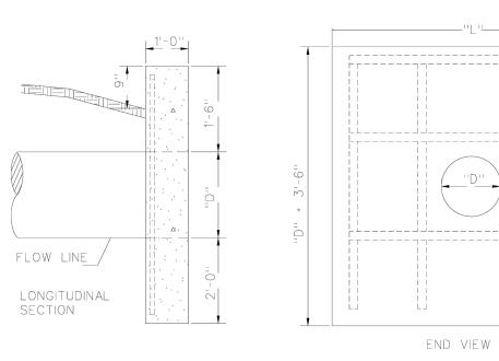
REINFORCED CONCRETE HEADWALL
